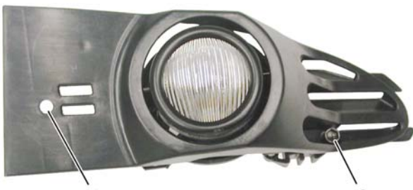
Mounting screw location
